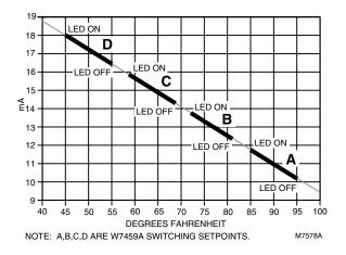
Fig. 3. C7650A Temperature Sensor Output Current.
